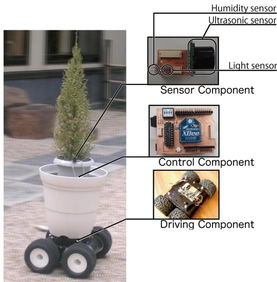
**Figure 3. The PotPet prototype.**
