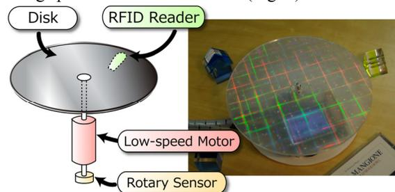
**Figure 2.** The prototype IODisk.
